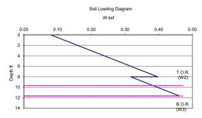
Horizontal lines indicate top & bottom of riser wall
