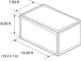
**Vault Isometric View** (Joints not shown for clarity) (All dimensions I.D.)
