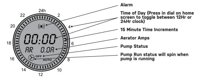
Elapsed time meter and cycle counter for pump and aerator included. To toggle between ETM and CC, press in the dial when on pump or aerator counter screens.
