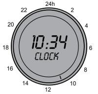
To set Timer, turn dial until Timer 1 is displayed, press in for enter, turn dial to the correct start time, press in dial, turn dial to the correct stop time, press dial.
