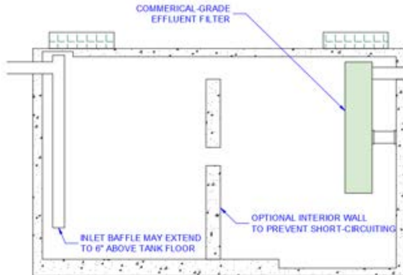
Figure 5—Grease Trap (Example Tank Only - Consult with FujiClean distributors for local regulation details)
